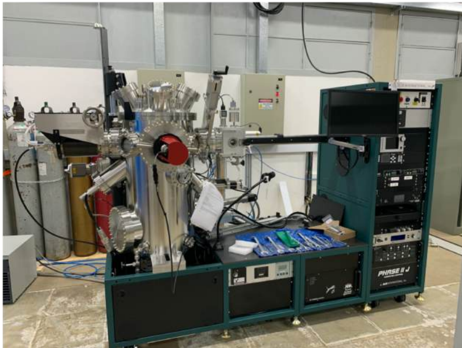
Figure 4.1: Top) LABNANO CBPF, photo lithography system Heilderberg DWL 66+. Bottom) LFDQ IFGW AJA Magnetron sputtering and angled e-beam deposition system.
