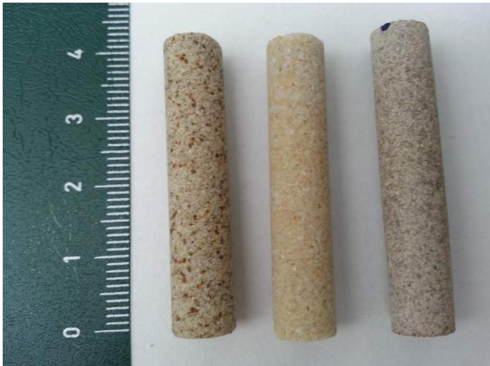
Figure 4.7.: Outcrop rocks used in high-field NMR experiments. From left to right is the Buff Berea Sandstone, Berea Sandstone and Indiana Limestone.
