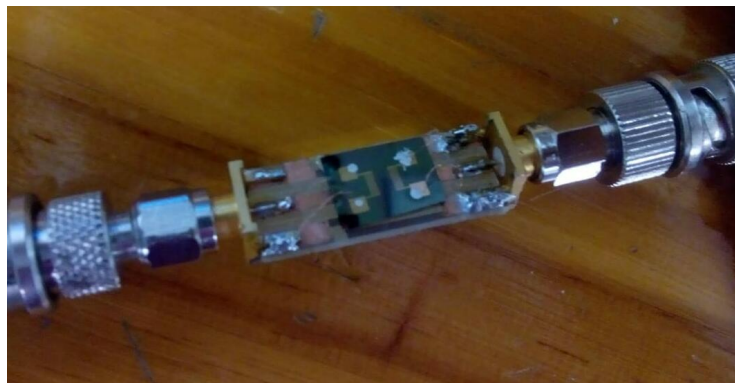
Figure A.9: The experimental IdTs electrical transmission setup. The input IdT is connected to a RF signal generator, and the output IdT, to a rectifying diode and a DC voltmeter.
