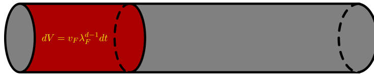
Figure 2.14.: Volume element for a quantum particle propagating with velocity v_F , in a tube of radius \lambda_F , during a time interval dt .
