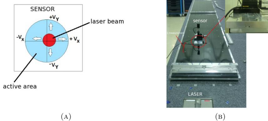
FIGURE 7.12: In (A) an illustration of the sensor working principle. In (B) the experimental setup to measure the alignment pins on fibre mat. The support for the sensor with the cavity to allow the passage of the pins is highlighted.
