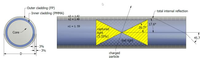
FIGURE 7.3: Transverse (left) and longitudinal (right) section of a double cladded fibre, with a schematic representation of the light generation and transport [93].
