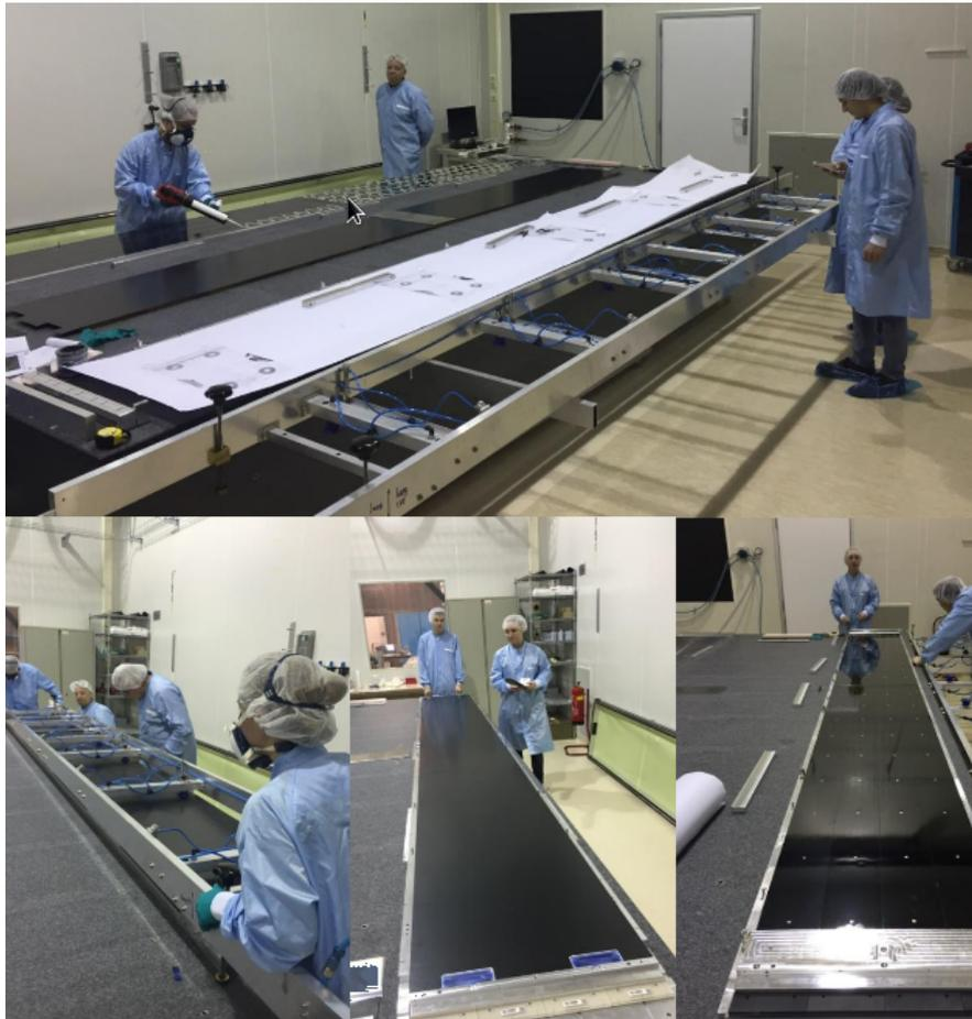
FIGURE 7.11: The photo on top shows the glue being applied to the surface of the 8 mats. Bottom left, the panels on top of the mats pressed with vacuum bump. Bottom right shown the bonded half-module turned, where after the quality test the second half-panel must be glued.
