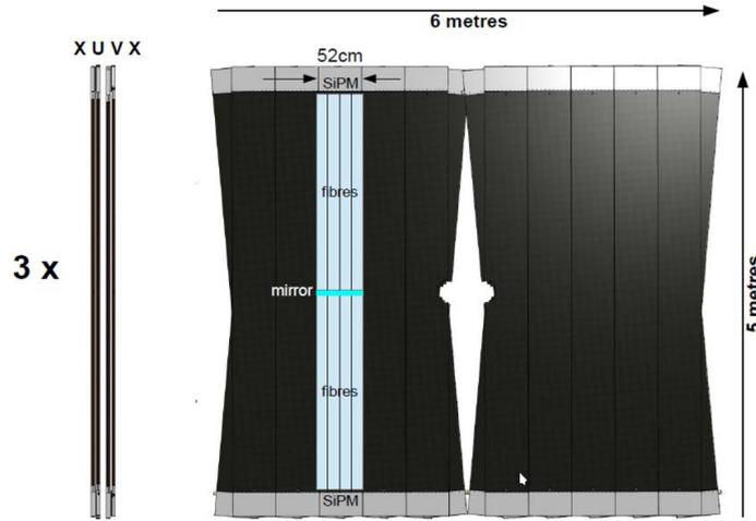
FIGURE 7.2: Schematic view of the SciFi Tracker. Highlighted in blue are the eight fibre mats with the mirror in the middle. Mirrors are glued to the end of the fibres mats to increase the light yield.
