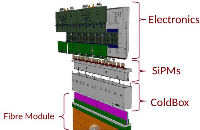
FIGURE 7.5: Schematic view of the SciFi layer composed of a module, cold-box, 16 SiPMs and the read-out electronics.
