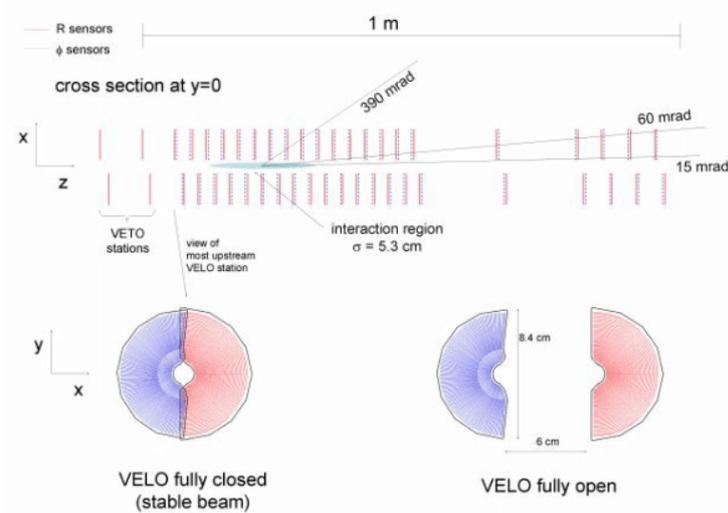
FIGURE 3.6: Cross-sections of the LHCb vertex locator. On top is the top view in the  $yz$ -plane of the VELO sensors, in red lines are the R sensors and blue lines are  $\phi$  sensors. On bottom the  $xy$ -plane views of the first two modules in both closed (left) and open (right) positions [38].
