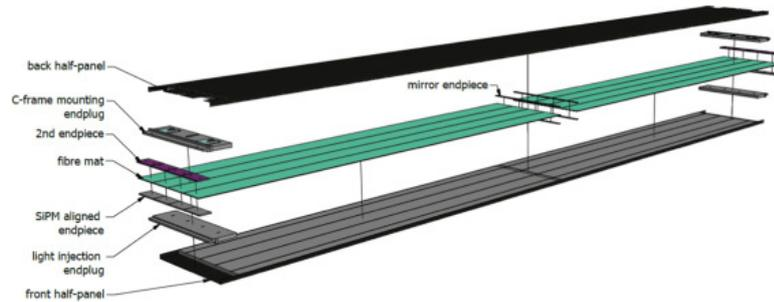
FIGURE 7.10: Schematic illustration of all fibre module components.
