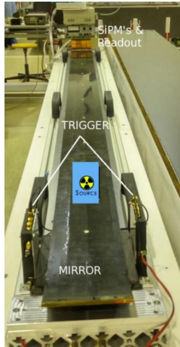
FIGURE 7.8: Setup to measure the light yield of a fibre mat.
