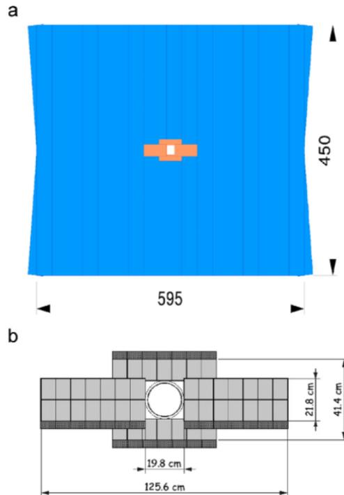
FIGURE 3.8: On top a layout of the OT station, with IT station in the centre region. On bottom a layout of the IT station, which is surrounded by the beam pipe and covered by silicon strip detector [44].
