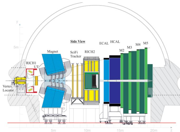
FIGURE 7.1: Schematic side-view of the upgraded LHCb detector, where UT stands for Upstream Tracker (the current TT station). and SciFi Tracker for Scintillating Fibre Tracker (the current T-stations) [92].
