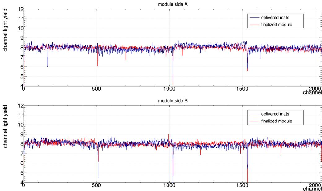
FIGURE 7.15: Light yield measured with cosmic rays for a full size detector module. Side A measurement corresponds to the four fibres mats placed of the top of the module while Side B measurement correspond to fibres mats of the bottom of the module. In both measurements, the light yield is homogeneous with no apparent damages.
