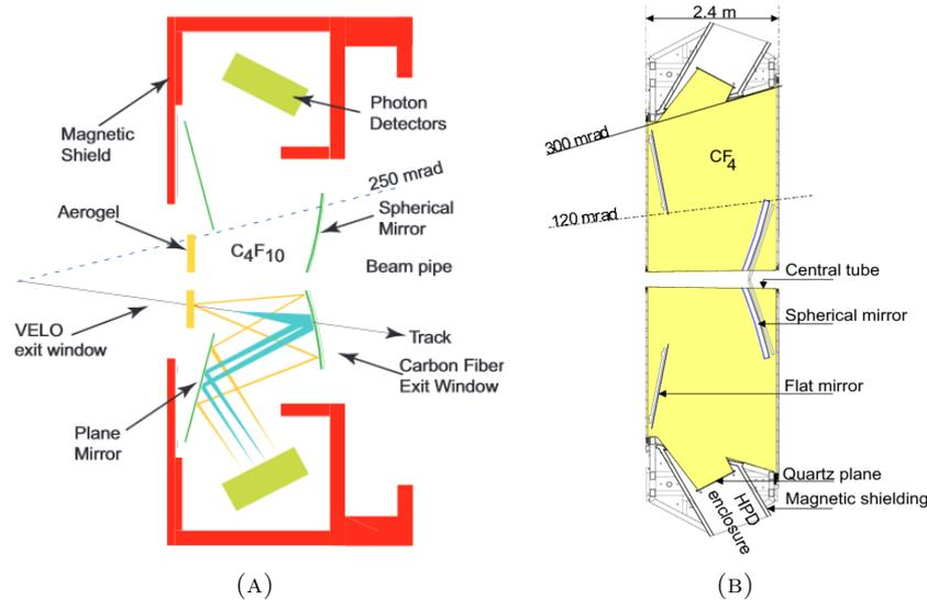
FIGURE 3.9: (A) schematic layout of the RICH 1 detector and (B) top view schematic of the RICH 2 detector [38].
