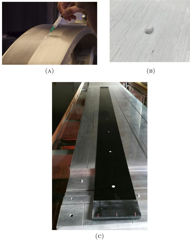
FIGURE 7.7: (A) pin hole being filled with glue in the winding wheel, (A) pin hole on fibre mat and (C) a finished fibre mat, where in white are the alignment pins.
