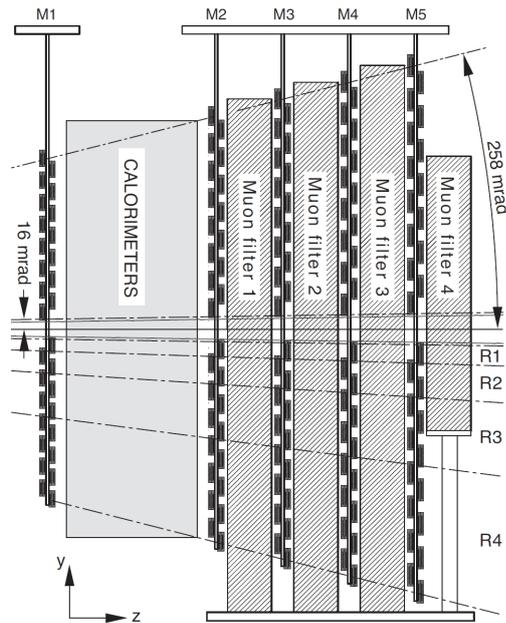
FIGURE 3.11: Schematic figure of the LHCb muon detector showing the five stations M1-M5 [38].
