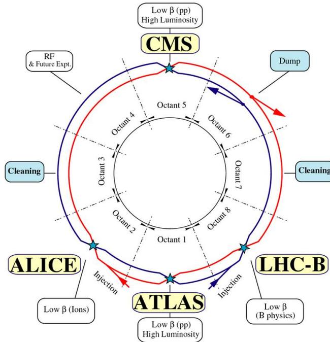
FIGURE 3.1: Schematic layout of the LHC and positions of the four main experiments [36]
