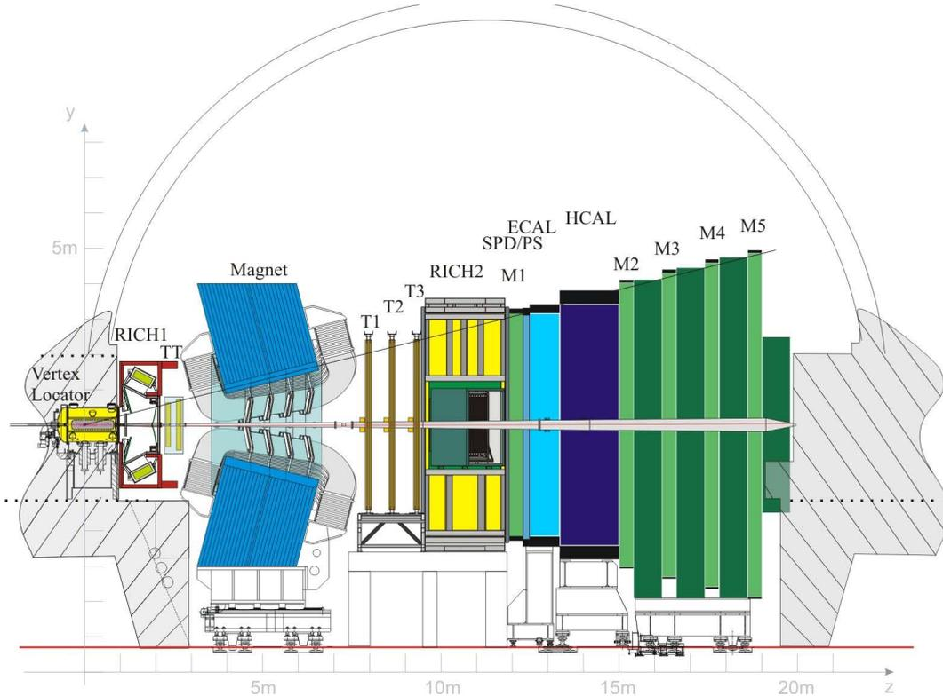
FIGURE 3.3: Schematic layout of the LHCb experiment [38].
