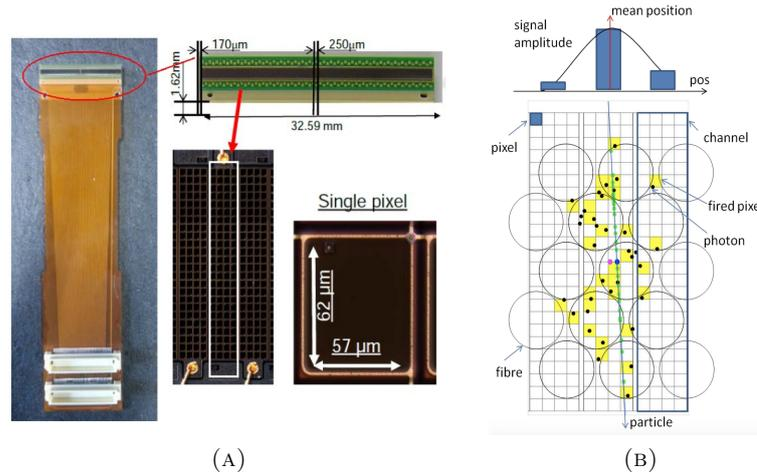
FIGURE 7.4: In (A) overview of one silicon photomultiplier. The elpise denotes the 128 channels and the white rectangle shows one channel. In (B) the detection principle of the SciFi tracker. The fibres cross-sections are indicated in blue. The fired pixels are highlighted in yellow. Taken from [89].
