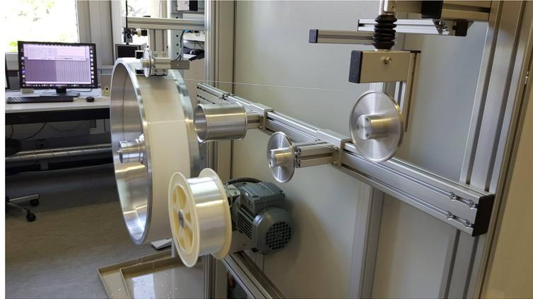
FIGURE 7.6: The winding machine which is used to lay and glue the 6 layers of fibre.
