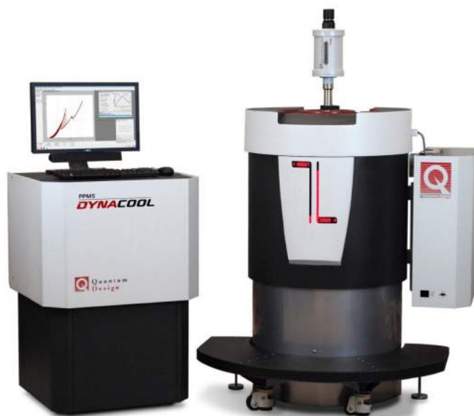
Figura 4.14 – PPMS Dynacool, Quantum Design, com módulo VSM ( Vibrating Sample Magnetometer ). Fotografia reproduzida da Ref. [187].
