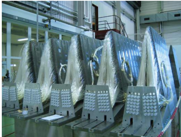
Figura C.3: HF wedges during assembly and the longitudinal quartz fibers with the light guides[169].
