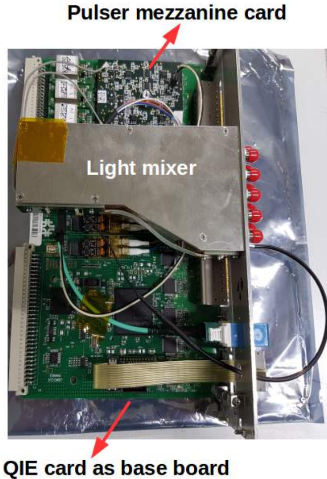
Figura C.9: HF calibration unit. The additional components are exhibited: the pulser mezzanine card and the light mixer.
