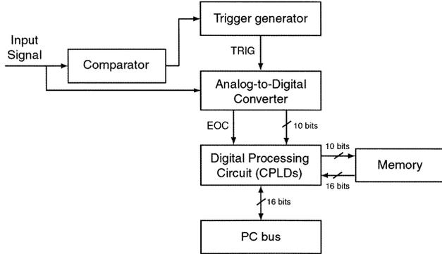
Fig. 1. Block diagram of the MCA circuit.
