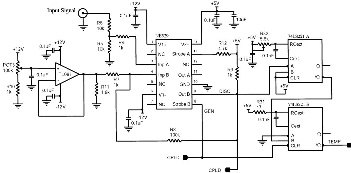
Fig. 2. Comparator and trigger generator circuits.
