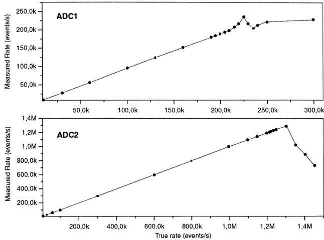
Fig. 4. Maximum counting rate of the MCA for both ADCs tested.
