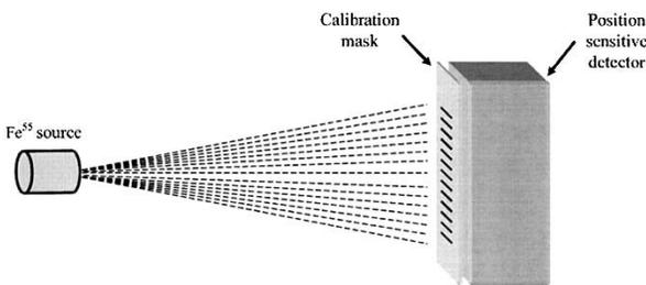
Fig. 8. Experimental setup for the integral nonlinearity measurement.
