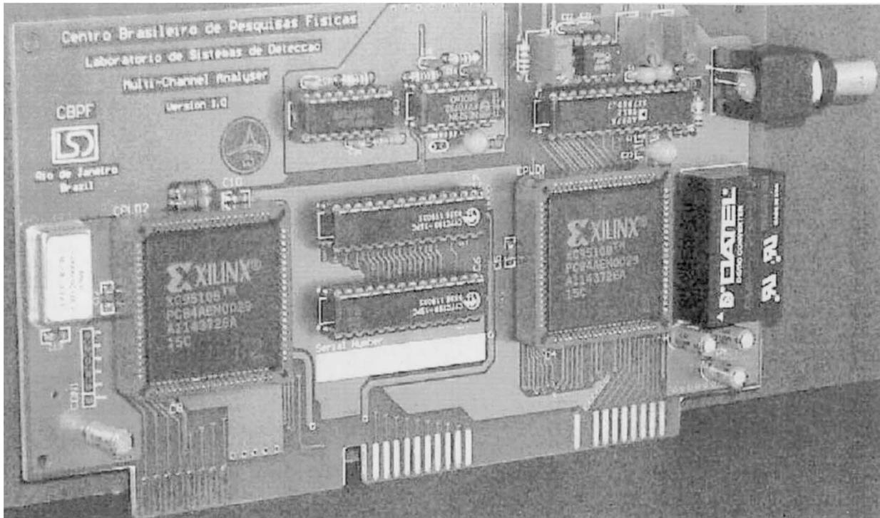
Fig. 11. Printed circuit board for the presented MCA.
