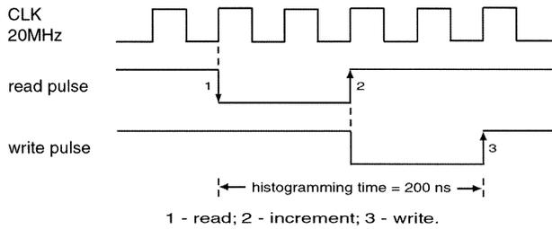
Fig. 3. Timing diagram for the state machine.
