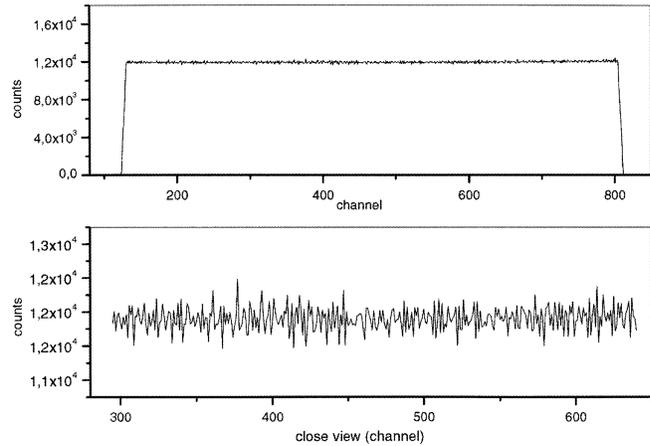
Fig. 5. Homogeneity histogram using a TAC and two-signal generators to generate the input signal.
