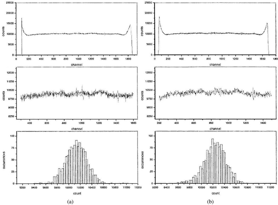
Fig. 7. Homogeneity spectrum for (a) the developed MCA and (b) for a commercial one.
