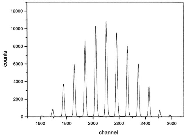
Fig. 9. Peak profiles resulting from the illumination of the detector through a calibration mask.
