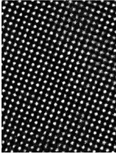
Figure 20: Atomic resolution HREM of a rutile \text{TiO}_2 (0,0,1) plane.
