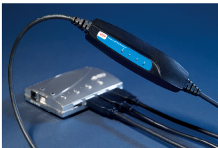
Figura 7: Interface CAN – USB comercial – Kvaser Leaf HS.
