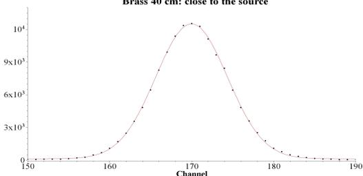
**Fig. 6: 0.40 m brass rod touching the source**
