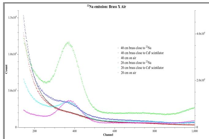
**Brass Experiments** - Concerned with the eventual deformation of the spectra shapes resulted from the  $\gamma$ -rays interactions in metals and how it could interfere in the final results, some other complementary tests were also performed. It is well known that  $\gamma$ -rays strongly interact with the MM they are crossing. In this way, taking
