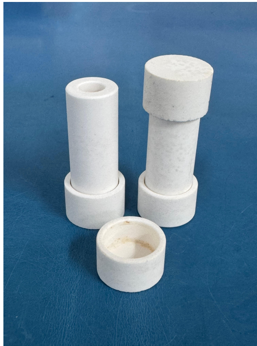
Figure 3.1: High alumina-based ceramic cylindrical molds with diameters of 7.5 mm and lengths of 38 mm , respectively, used for sample preparation in experimental procedures.
