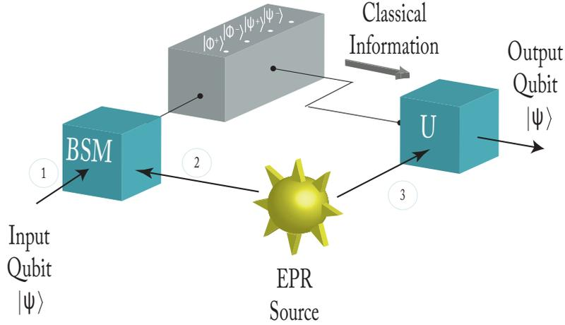
Figure 6.7: Schematic diagram of an arrangement for teleportation and Bell measurement.
