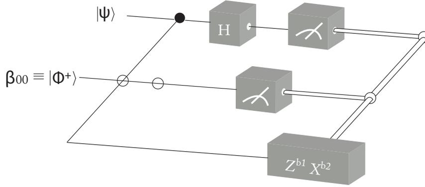
Figure 6.6: Complete quantum circuit for the teleportation process.
