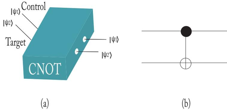
Figure 6.2: Schematic diagram of a C-NOT gate.
