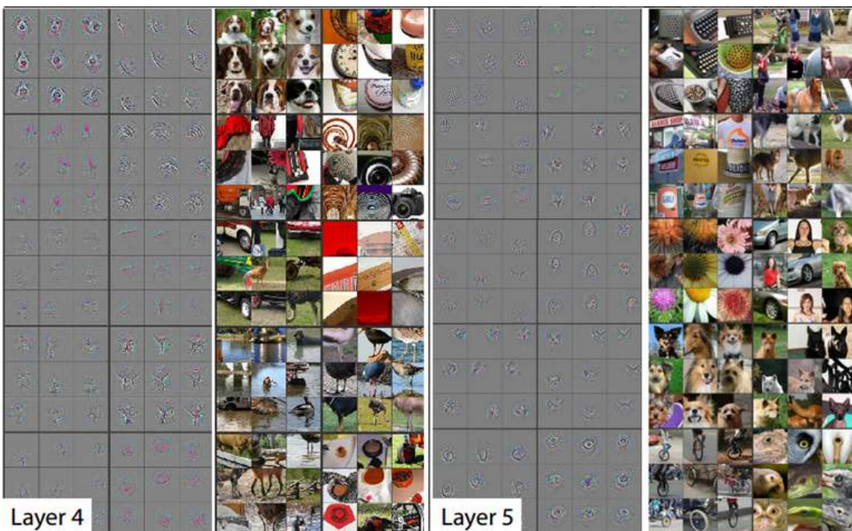
Figure A.4 – Visualizations of some examples of images for different classes used in the ZF-Net and the structures of these images that produce the greatest activations of the net. Source: Zeiler and Fergus (2014).
