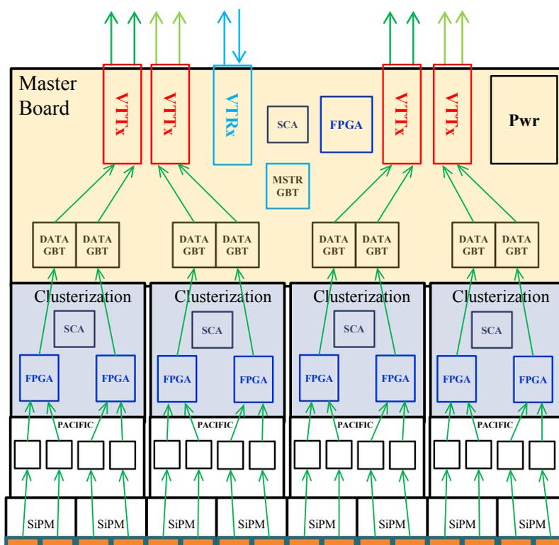
**Figure 1.** Block Diagram of half a ROB. The main components on each board are shown. The data flow is denoted by the green line.
