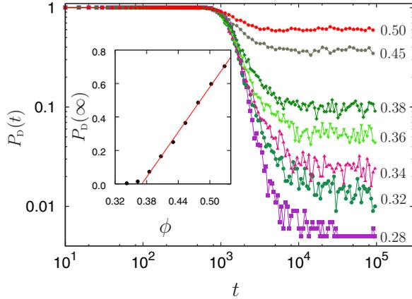
FIG. 4. (Color online) Probability of percolation of D clusters as a function of time,  $P_D(t)$ , for several area fractions  $\phi$  and the same parameters as in Fig. 2. Inset: Asymptotic limit of  $P_D(t)$  as a function of  $\phi$ . The linear fit indicates that the percolation probability goes to 0 at  $\phi \simeq 0.37$ . The small deviation seen close to this point is due to the long time of convergence.
