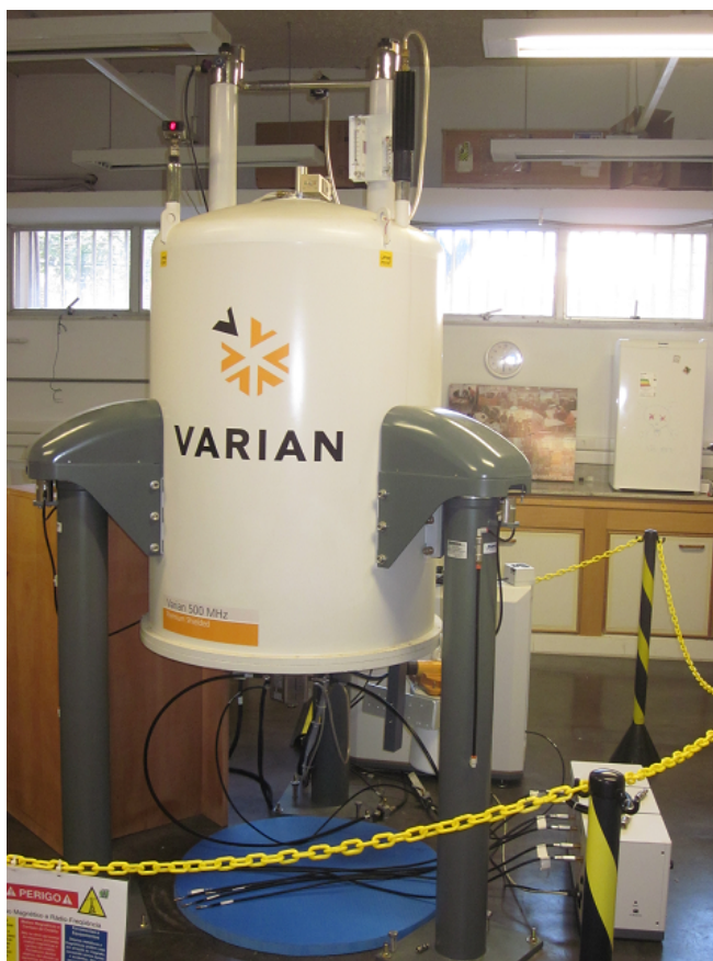
Fig. 2.22: Varian 500 MHz NMR magnet. The fill ports for liquid Nitrogen and Helium are at the top of the magnet. The probe is inserted at the bottom of the magnet, while the sample is inserted from the top.
