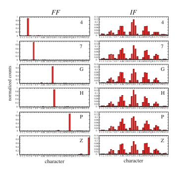
FIG. 4 (color online). Normalized counts for Bob's Fourier (*F*) detection system when Alice uses Fourier (left) and image (right) encoding.
