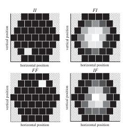
FIG. 3. Intensity distributions at Bob's detection plane for the four lens configurations *II*, *IF*, *FI*, and *FF* for the case when Alice sends the character 7. Here lighter squares correspond to a larger number of photocounts.
