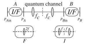
FIG. 1. Illustration of QKD using imaging (I) and Fourier (F) optical systems.
