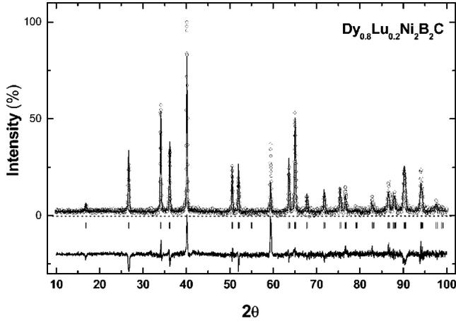
FIG. 1. Room temperature x-ray diffraction pattern of the  $\text{Dy}_{0.8}\text{Lu}_{0.2}\text{Ni}_2\text{B}_2\text{C}$  sample. The structural and conventional Rietveld parameters are shown in Table I.
