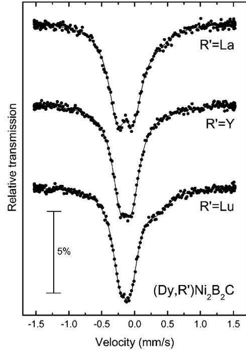
FIG. 2. Room temperature  $^{57}\text{Fe}$  Mössbauer spectra of  $\text{Dy}_{0.8}\text{R}'_{0.2}\text{Ni}_2\text{B}_2\text{C}$  ( $\text{R}'=\text{Y}, \text{Lu}$ ) and  $\text{Dy}_{0.92}\text{La}_{0.08}\text{Ni}_2\text{B}_2\text{C}$ .
