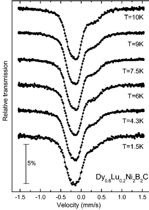
FIG. 3.  $^{57}\text{Fe}$  Mössbauer spectra of  $\text{Dy}_{0.8}\text{Lu}_{0.2}\text{Ni}_2\text{B}_2\text{C}$  for  $1.5 \text{ K} \leq T \leq 10 \text{ K}$ .
