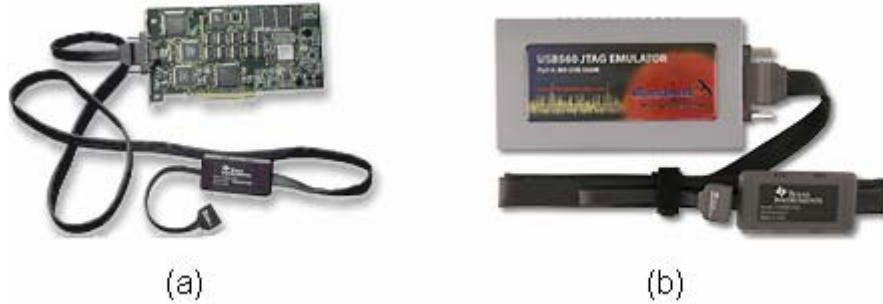
FIGURA 5: EXEMPLO DE EMULADORES JTAG [2]. (A) XDS560 PCI-BUSSS JTAG SCAN-BASED EMULATOR (DSP8032U). (B) BLACKHAWK XDS560 USB EMULATOR (DSP11990U)
