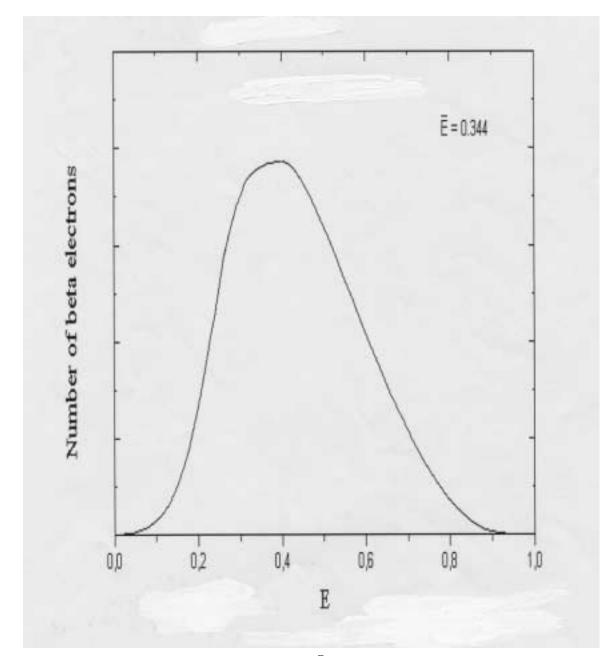
the measured value was  $0.344(\pm 10\%)MeV = \overline{E}$ . The possible gamma-rays which would be emitted together with the electrons (and not absorbed in the calorimeter) and account for the missing energy, were shown by Meitner – with counters – not to exist.
