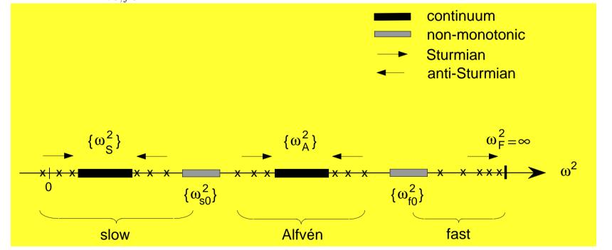
• Oscillation theorem: Outside  $\{\omega_{A,S}^2\}$ ,  $\{\omega_{s0,f0}^2\}$ , the discrete spectrum is monotonic in number of nodes of eigenfunctions (either Sturmian or anti-Sturmian).
