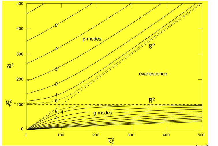
• Frequencies *p*-modes *increase* monotonically, clustering at  $\infty$ :  $\omega_p^2(q^2) \uparrow \omega_P^2 = \infty$ . Frequencies *g*-modes *decrease* monotonically, clustering at 0:  $\omega_g^2(q^2) \downarrow \omega_G^2 = 0$ .
