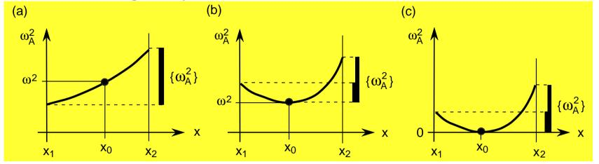
Case (a): If  $\omega_A^2(x)$  is monotonic, any  $\omega^2$  in the range  $\omega_A^2(x_1) \le \omega^2 \le \omega_A^2(x_2)$  leads to a singular point  $x_1 \le x_0 \le x_2$ , where the Alfvén factor may be expanded:
