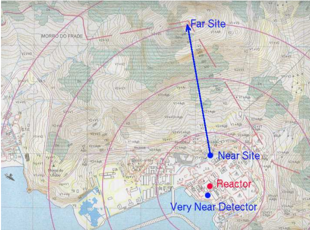
FIG. 1: Map of the Angra site, where the positions of the reactor, VND, ND and FD are indicated. The solid line indicates the horizontal tunnel to be excavated to give access to the far detector experimental hall, under the Morro do Frade peak. The solid circles indicate the distance from the Angra II reactor in 500 m steps.
