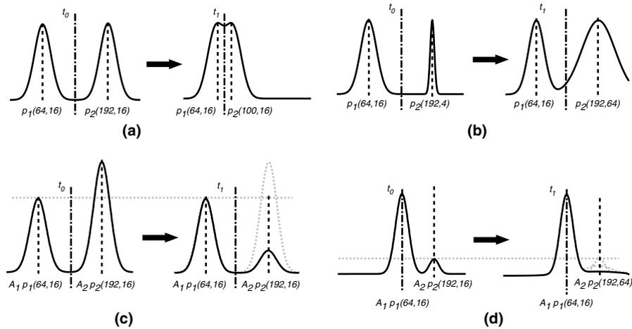
Fig. 1. Four gray level segmentation testing schemes: (a) peak position; (b) peak width; (c) peak height and (d) noisy image. We define a position and a width for each peak.
