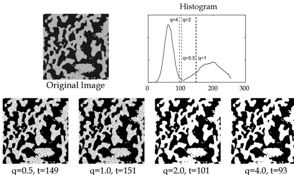
Fig. 5. Example of nonextensive entropic segmentation. Image of a magnetic domain structure with a regular spatial noise. Result of segmentation for  $q = 0.5, 1.0$  (classical entropic segmentation), 2.0 and 4.0.
