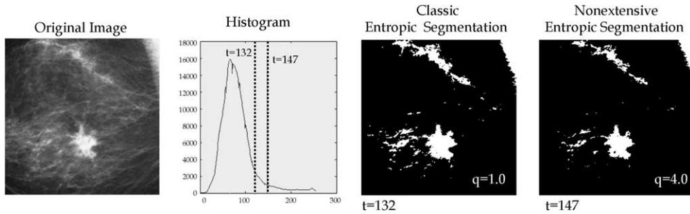
Fig. 3. Example of entropic segmentation for mammography image with an inhomogeneous spatial noise. Two image segmentation results are presented for  $q = 1.0$  (classic entropic segmentation) and  $q = 4.0$ .
