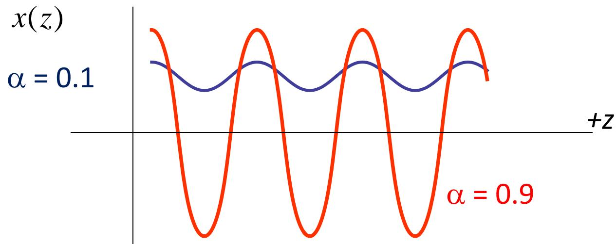
$$x(z) = \frac{\alpha}{k_u} \ln \left[ \frac{\alpha \cos(k_u z) + \sqrt{1 - (\alpha \sin(k_u z))^2}}{1 + \alpha} \right] \quad \alpha = \frac{a_u}{\gamma \beta}$$
